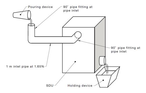
FIGURE B1 TYPICAL PAPER AND SOLIDS DISCHARGE TEST SET-UP
