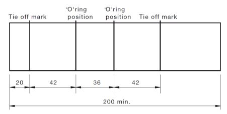
NOTE: Mark and cut off to length the natural or artificial sausage skin casing using this template.
