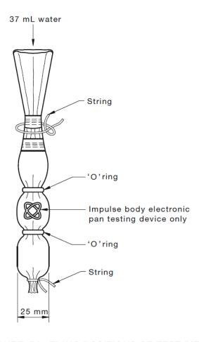
FIGURE B3 TYING POSITIONS OF TEST PIECE
